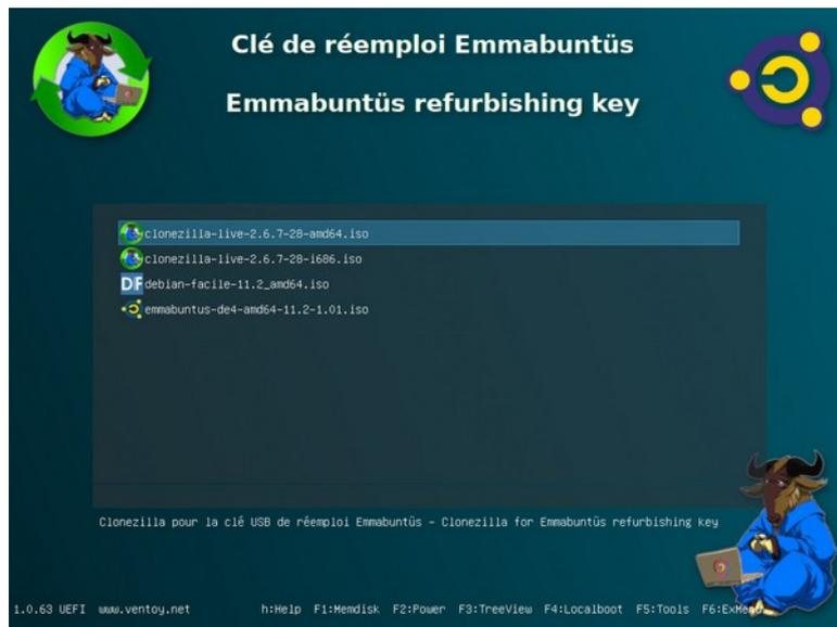
In the above window, you can run the reuse script with either 64-bit or 32-bit Clonezilla, and you will get one of the windows below to run the cloning script :
